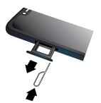
2 Insert the nano SIM first with the gold contacts facing down.
